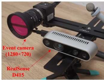
Fig. 4: Dual-camera setup. The left device is an event camera with resolution 1280 \times 720 . The right RGB-D camera is a RealSense D415, only used for evaluating base-line algorithms and doesn't form an input to our algorithm.
