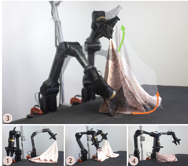
Fig. 1: Our system flips garments right-side-out with three keypoint-conditioned bimanual primitives: (1) DRAG exposes a single-layer hem; (2) FLING brings the single layer to the top; (3) INSERT&PULL grasps the interior and pulls through; (4) final right-side-out state.
