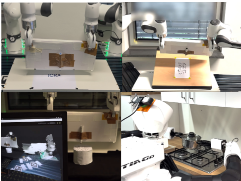
Fig. 4: The real-world experimental setup involves two Franka robots collaboratively grasping a pen for stippling operations and a TIAGo to carry objects using both hands.
