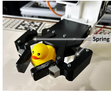
Fig. 5: Hand gripper with self-adaptive mechanism.
