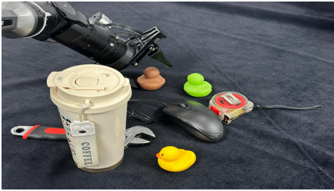
Fig. 6: Real-world experimental setup: Piper robotic arm paired with a Realsense camera.
