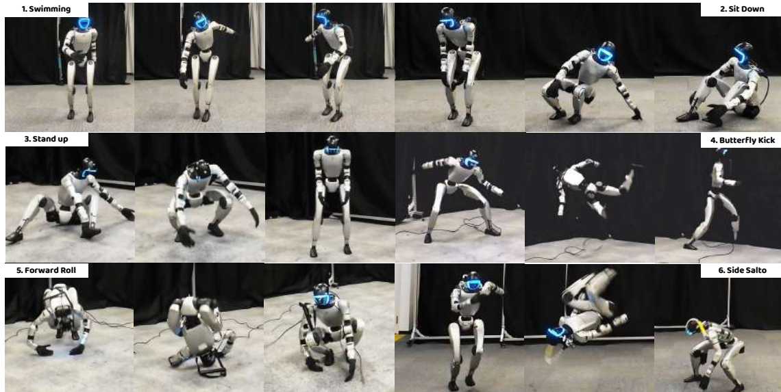
Fig. 1: Behavior Foundation Model enables humanoid robots to perform a variety of behaviors in a zero-shot manner, including (1) a swimming pose, (2) sitting down on the ground, (3) standing up from the ground, and (4) butterfly kick. It also facilitates efficient acquisition of new behaviors such as (5) a forward roll and (6) a side salto.
