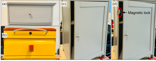
Fig. 3. Real-world articulated objects used in our experiments: (a) Drawer 1 without a lock, (b) Drawer 2 with a magnetic lock, (c) Door 1 without a lock, and (d) Door 2 with a magnetic lock.
