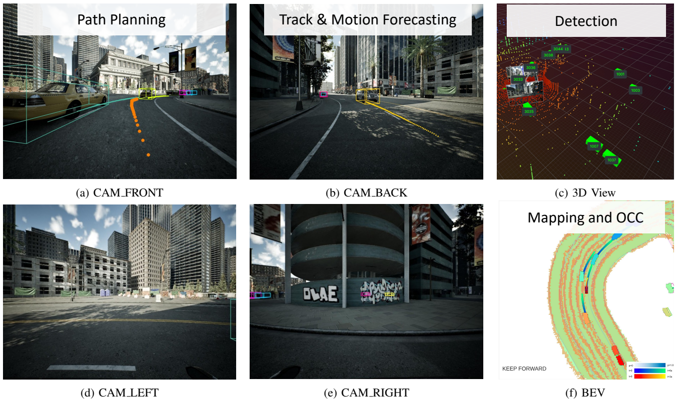
Fig. 1: Illustrations of various autonomous driving tasks using the M 3 CAD dataset. (a) Demonstrates the path planning (PP) results, where the ego vehicle’s predicted trajectory is represented by a dotted line. (b) Shows object tracking (OT) and motion forecasting (MF) results where dotted lines represent predicted trajectories of other vehicles. (c) Presents object detection (OD) results in 3D space. (f) Depicts mapping (MP) and occupancy prediction (OCC) results.
