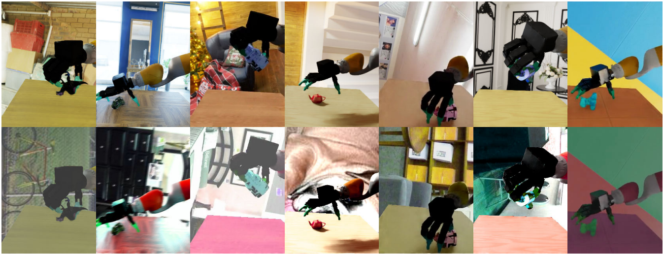
Fig. 4: The top row shows the left camera renderings for different environments in simulation. The bottom row shows various data augmentations applied to these sim renderings that are passed to the student policy.
