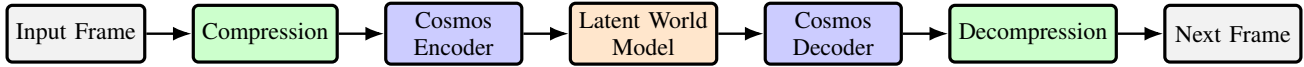
Fig. 3: Model pipeline: Input frame from video feed is optionally compressed, tokenized by Cosmos, propagated through a latent world model, decoded by Cosmos, optionally decompressed, and reconstructed into the next frame.
