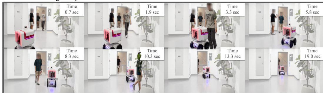
Fig. 4: Real-world elevator co-boarding experiments with human participants. (A) Single policy across diverse scenarios. (B) Scenario involving multiple human interactions.
