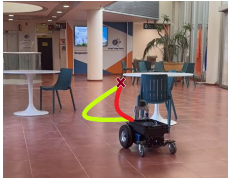
Fig. 9: ■ APPLR, ■ RL+OE. APPLR takes an exaggerated curve around a static obstacle, while RL+OE deviates less.
