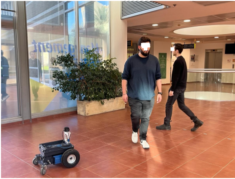
Fig. 1: RoverZero robot used in our real-world experiments; equipped with LiDAR and Odometry sensor.
