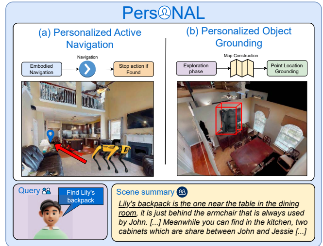
Fig. 1. We introduce PersONAL, a comprehensive benchmark to evaluate Embodied AI agents in the context of user-centric tasks. PersONAL supports two evaluation modes: (1) active navigation in unseen environments, and (2) object grounding in previously mapped scenes.
