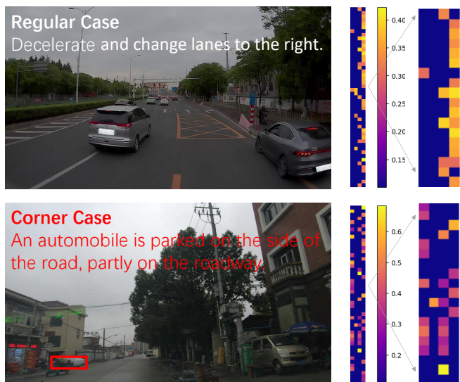
Fig. 3. The activation status of MoE is presented when the model encounters regular cases and corner cases. When encountering regular cases, the activation pattern of experts is relatively single. When encountering corner cases, more experts are activated.
