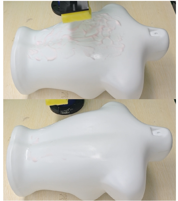
Fig. 8. Qualitative experiment of wiping task on the back of a human model in the real world. The top image shows the back before wiping, with pink foam indicating the area requiring cleaning. The bottom image shows the back of the human model after cleaning.
