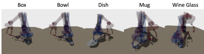
Fig. 5. Example successful grasping trajectories using our method; robot motion progresses from red to blue.
