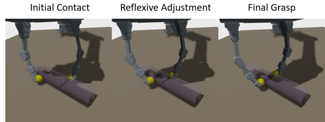
Fig. 1. A representative example of our reflexive grasping controller starting from an imprecise initial gripper configuration. The dashed line connects the two contact points, the black arrows indicate the contact normal vectors, and the arcs represent the angles between them – smaller angles indicate more stable grasps.
