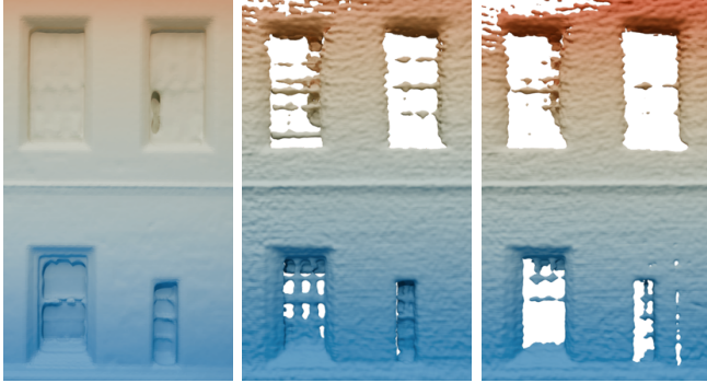
Fig. 3. Comparison of shadow models on the Newer College dataset (frames 1–250, voxel size 2.5 cm). Left: ground-truth reconstruction of the Quad at 1 cm resolution. Center: hemispherical model. Right: conical model.
