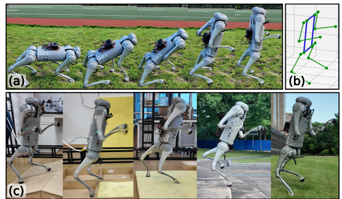
Fig. 9: (a) Transition from the walk skill to the biped skill. (b) Keyframe for the biped skill used for imitation. (c) Snapshots of executing the biped skill to traverse various indoor and outdoor terrains.
