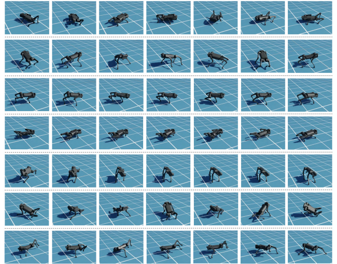
Fig. 3. Motion sequences of various skills. Each row illustrates the motion sequence corresponding to a distinct skill, with the robot performing movements at a specific velocity and posture.
