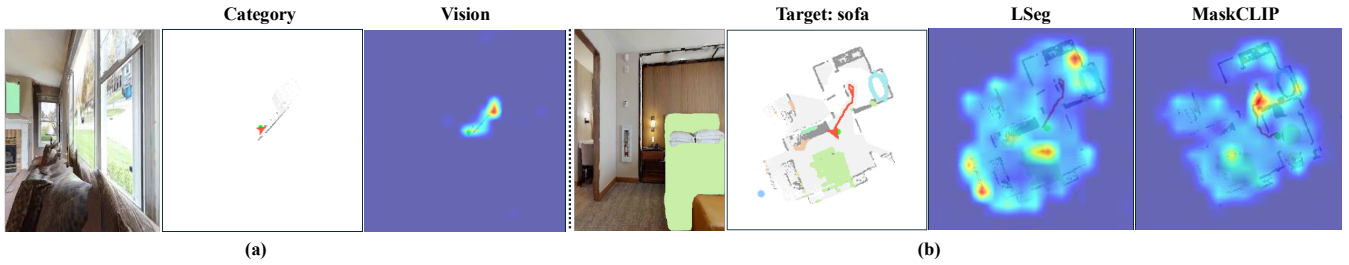
Fig. 3. (a) When detection fails, the text-based map lacks context, while the vision-based map remains robust with richer information. (b) In the self-attention layers, LSeg focuses more precisely on relevant objects, while MaskCLIP’s attention is more dispersed.
