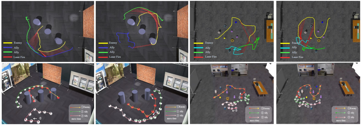
Fig. 6: The first row shows the trajectories of robots in the laser tag game in simulation. When the firing condition is met, an ally robot fires a laser beam toward the enemy, indicated by the red line. The second row shows the robot motions, with enemies in red and allies in white. Allies maneuver strategically to aim and attack the enemies, while the enemy maneuver to escape.
