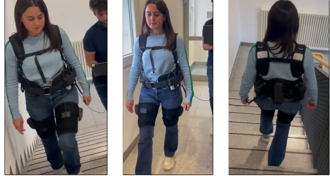
Fig. 1. We equip an easy-to-wear and light exosuit with a user-tailored perception model estimating the current and intended walking gait (ascending or descending stairs and walking on level ground) using only IMU readings.
