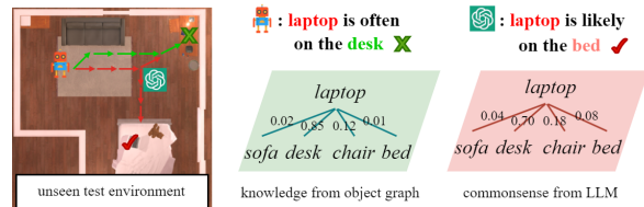
Fig. 1. In the training environment, the agent learns that a laptop is often on the desk, leading to incomplete or incorrect knowledge in the object graph (middle). However, in an unseen test environment (left), the laptop may instead be located on the bed. Commonsense knowledge extracted from the LLM correctly predicts that a laptop can also be on the bed (right), helping the agent to find the laptop.
