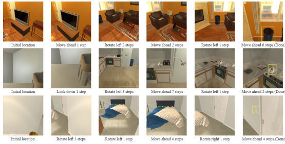
Fig. 7. Visualization of the agent’s first-person view in AI2-Thor. The target objects found by the agent are marked by yellow boxes.
