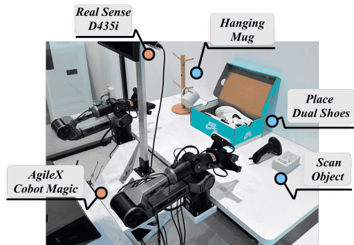
Fig. 6. Real-World Experimental Setup. Our experimental setup consists of an AgileX Cobot Magic dual-arm robot equipped with a RealSense D435i head-mounted camera.
