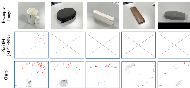
Fig. 6. Qualitative Results. SfM with our method is qualitatively compared with the detector-based baseline PixSfM on Texture-Poor SfM Dataset.
