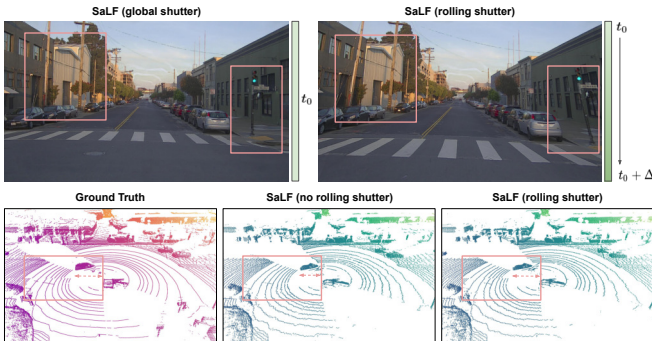
Fig. 10. Rolling-shutter simulation via SaLF-Ray. Top: We render the same view using global shutter and rolling-shutter camera models (see highlighted distorted region). Bottom: SaLF simulates rolling-shutter effect and accurately match ground truth point clouds (see lidar sweep seam and relative position for the dynamic actor.)
