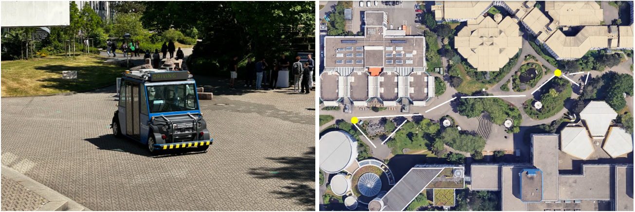
Fig. 2. Real-world experimental setting showing the AutoBus with the 'DRIVING' visual cue displayed on its front LED screen (left), and a top-view snapshot of the 480-meter experimental route on campus (right).
