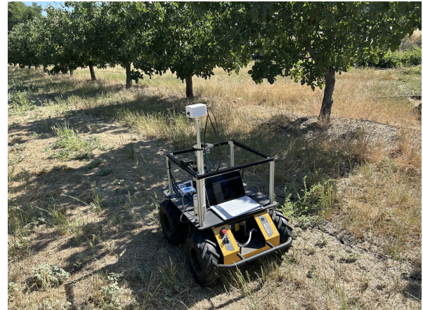
Fig. 1: A task in precision agriculture: a robot acquiring thermal imaging of a pistachio tree for water stress detection.
