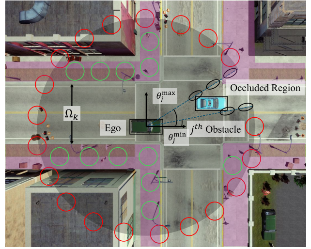
Fig. 2. Visualization of the GM components in the S-OA birth model. Black, green, and red components correspond to the occlusion-based terms (10), semantic-based terms (13), and boundary terms at the edge of the sensor's FOV (15), respectively.
