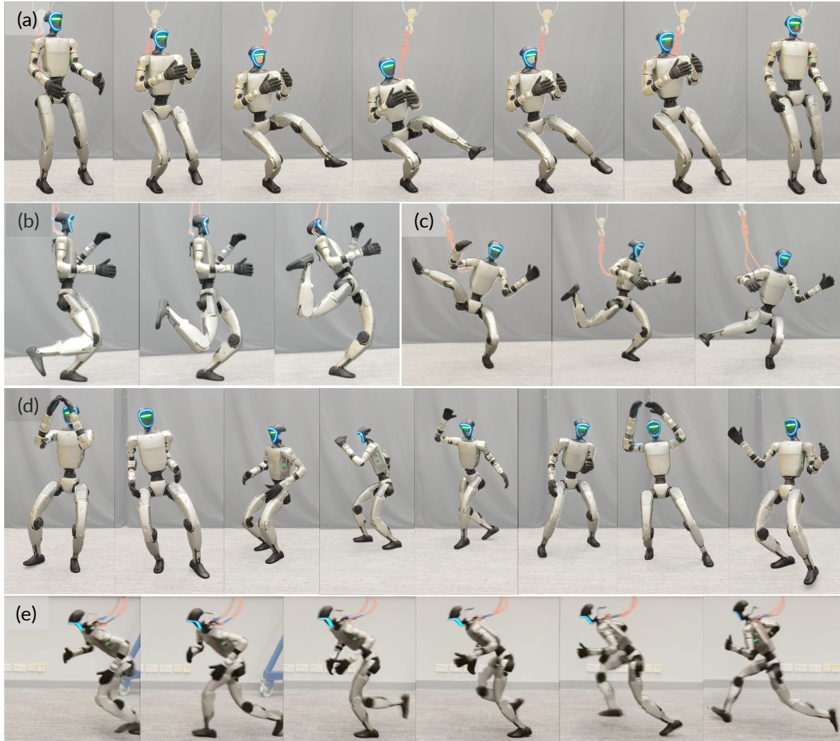
Fig. 1: Introducing AMS (Agility Meets Stability), one single policy that performs diverse motions with stability and agility simultaneously on a humanoid robot. The robot can execute challenging balance motions such as (a) Ip Man's Squat, a Kung Fu-style single-leg squat, unseen during training (zero-shot); (b) single-leg balance stances which humans find hard to perform; (c) balanced stretching; as well as expressive motions and high-mobility movements with precise control, such as (d) dancing and (e) running.
