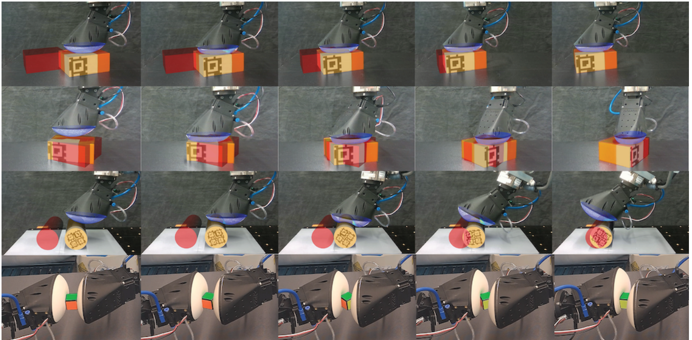
Fig. 6. Real-world experiments. Sequential frames illustrating the four manipulation tasks: planar pushing (top row), planar rotation (second row), rolling (third row), and in-hand rotation (bottom row). The orange outline indicates the object pose, and the red outline denotes the goal pose.
