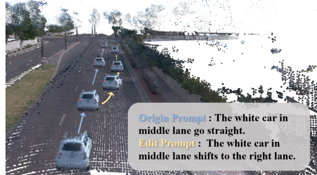
Fig. 1. The diagram of the proposed LangEditor. We use a text prompt to identify the object to be edited and determine the new trajectory, then modify the position of the vehicle within the scene for 4D editing.
