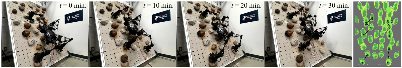
Fig. 10. Rock climbing with LIMBERO under full Earth gravity. The right foothold history indicates the initial grasping points (black dots) and the step order (numbers) on the graspability-assessed terrain map. The 7th step represents a regrasp action around the same foothold. Regions with very low graspability are omitted from the visualization.
