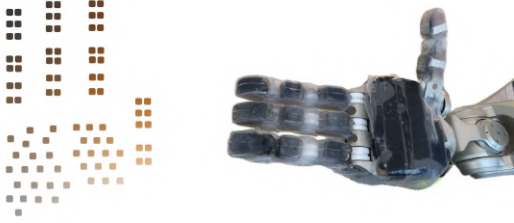
Fig. 2. Sensor array layout (left). Illustration of the sensor array covering the palm and fingers of the Meka M2 Robot hand (right).
