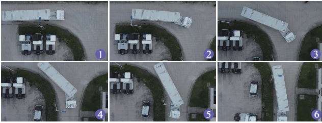
(b) A bird-eye view of an articulated truck making a right turn.
