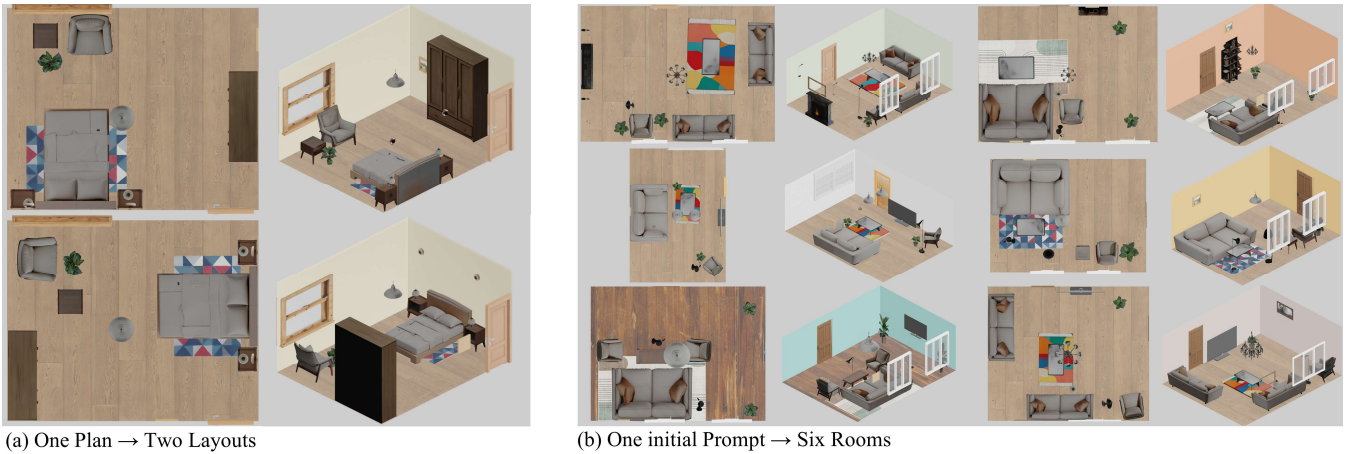
Figure 4. Our pipeline generates diversity from two distinct sources: physical placement and semantic generation. (a) Placement-level diversity: Two distinct layouts generated from a single, detailed semantic plan, demonstrating how the force-directed simulation finds multiple stable equilibria. (b) Semantic-level diversity: Six different living rooms generated from the single high-level prompt "living room", demonstrating the LLM's ability to first create varied semantic plans, with one resulting layout shown for each.
