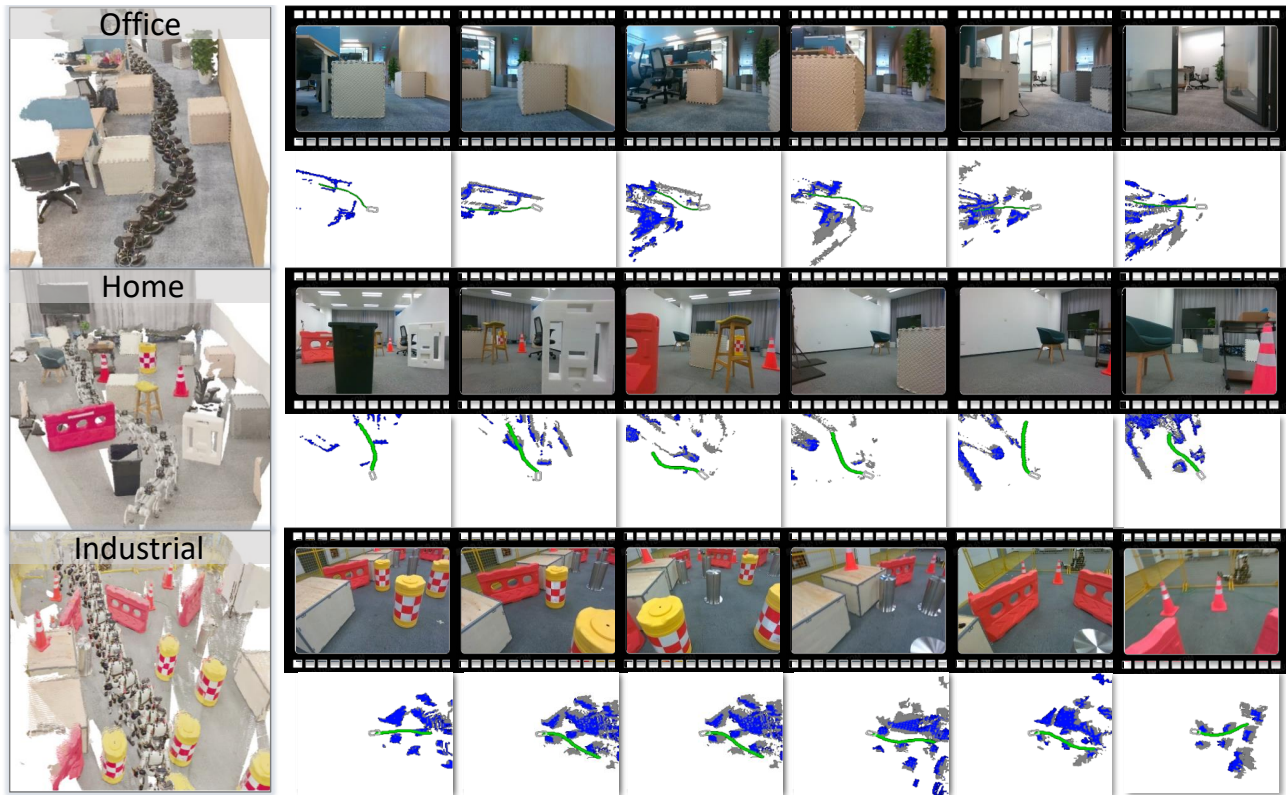
Fig. 4. Visualization of LoGoPlanner in real-world scenarios on different robot platforms. The green curves are the planned trajectories of LoGoPlanner. Blue and grey clouds are the obstacles of the current frame and the previous frame respectively.
