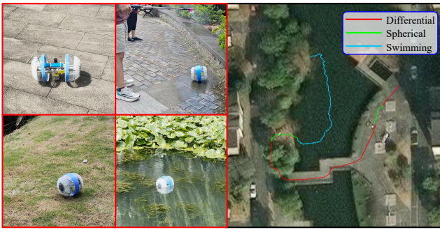
Fig. 7. Illustration of outdoor multi-terrain tracing. The movement track recorded by RTK-GPS on the right.
