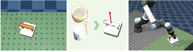
Fig. 5: Qualitative results on pickup kettle in MuJoCo with a UR5e manipulator. RAAP successfully transfers handle-oriented affordances to kettles.
