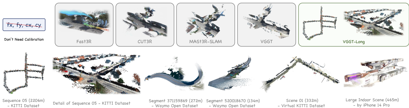
Fig. 1. For large-scale outdoor scenarios, previous work suffers from: 1) severe drift (CUT3R and Fast3R); 2) unable to complete the entire long sequence (MASt3R-SLAM and VGGT). Our method VGGT-Long is able to reconstruct the kilometer-scale scene while maintaining the accuracy of the scene.
