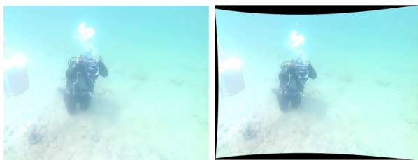
Fig. 6: An optical dataset image before and after correction of radial distortion using OpenCV camera calibration.
