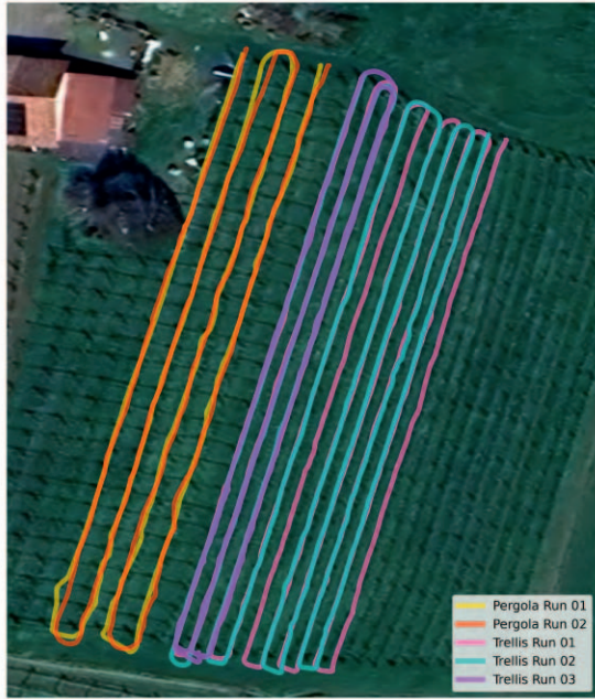
Fig. 4: Trajectories for the three runs conducted in the trellis vineyard and in the pergola vineyards, overlaid with the satellite image of the field.
