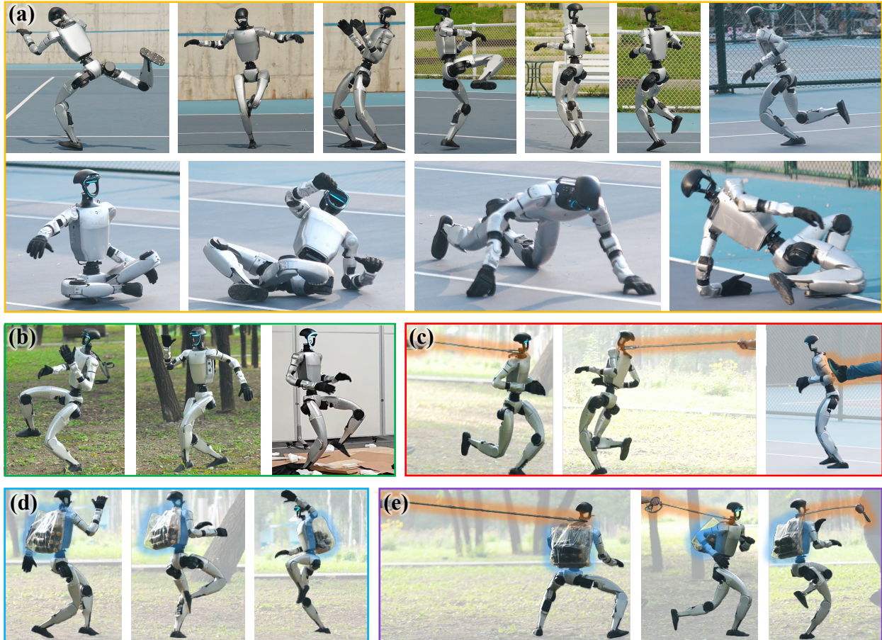
Fig. 1: (a) The humanoid tracks diverse, highly dynamic, and contact-rich motions using a single policy. (b) The humanoid tracks motions on different terrains . (c) The humanoid tracks motions against different external forces , including pulling forces from the rope and pushing forces from the human feet. (d) The humanoid tracks motions against physical property changes (the payload on the back). (e) The humanoid tracks motions against all dynamics disturbances , including terrains, external forces, and physical property changes simultaneously.
