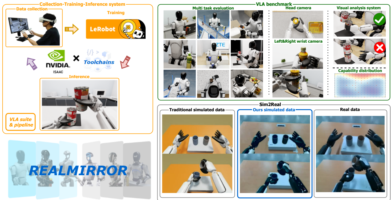
Fig. 1: The RealMirror framework for accelerating VLA research in humanoid robots. (a) Top-left: Our data collection, training, and inference system is developed based on VR teleoperation, Lerobot, and Isaac Sim. (b) Top-right: This platform populates a benchmark for humanoid robots with multiple scenarios and various VLA models. (c) Bottom-right: The striking photorealism of the simulation bridges the reality gap, enabling zero-shot Sim2Real transfer without any fine-tuning.
