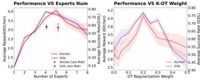
Fig. 6: Ablation studies. Left: Performance under varying numbers of experts in the MoE decoder. Circle markers denote single-model variants without MoE, placed at x-axis positions indicating the number of experts with roughly equivalent total parameter count. Right: Performance under different OT regularization weights.
