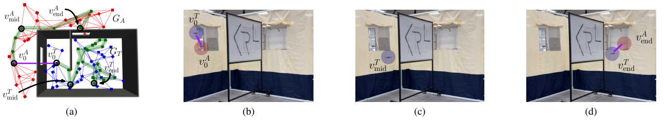
Fig. 1: (a) Illustration of motivating application where R_{\text{task}} (blue) and R_{\text{assist}} (red) need to maximize accumulated line-of-sight (LOS) (purple) while moving on their respective roadmaps G_T, G_A . Computed paths depicted in green. (b)-(d) Snapshots of path execution on Crazyflie drones for three timestamps t_0 = 0, t_{\text{mid}} and t_{\text{end}} = 1 where R_{\text{task}} and R_{\text{assist}} are located at v_0^T, v_{\text{mid}}^T, v_{\text{end}}^T and v_0^A, v_{\text{mid}}^A, v_{\text{end}}^A , respectively. As R_{\text{task}} is required to move between two parts of the room, R_{\text{assist}} needs to strategically reposition itself causing a temporary lack of LOS at t_{\text{mid}} (thus, v_{\text{mid}}^T is not visible in (b)).
