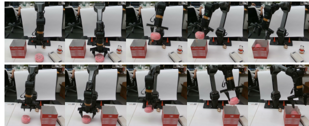
Fig. 5: Visualization of the real world experiments. The model is asked to place the pink ball into the box. We show two samples with different layouts and chaos background.
