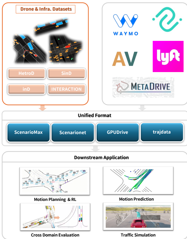
Fig. 5: We develop a unified development toolkit that converts a wide range of traffic scene datasets into standardized, agent-centric data formats [43], [44], [46], [47], enabling seamless comparisons across datasets for forecasting, planning, and simulation.
