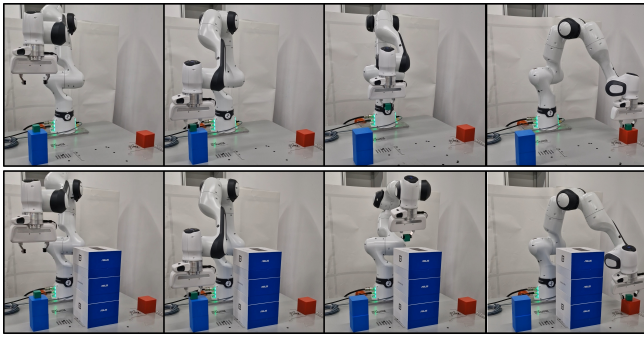
Fig. 5: Deployment on the Franka Research 3 for cluttered tabletop pick-and-place. Top: grasp at the first goal and place at the second. Bottom: with an obstacle, the controller lifts to avoid collision and completes the placement.
